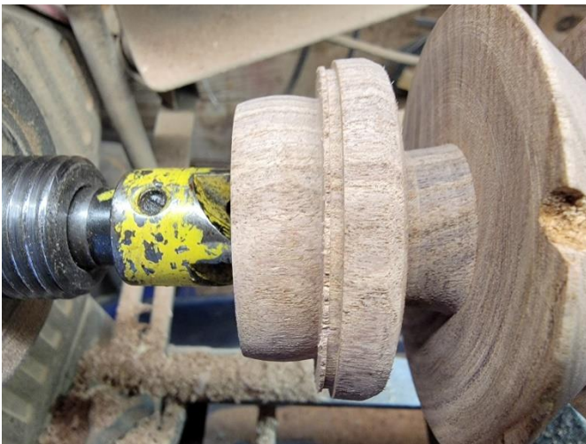
#5 Tenon is Beveled on Both Ends to Swivel in Chuck Jaws
