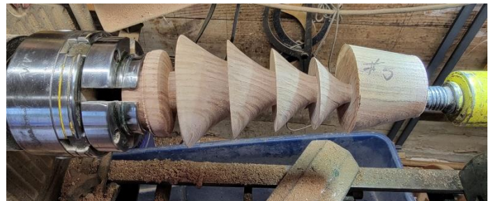
#10 Set Up on Point #5 Minimum turning required on the tip. Trying to turn the tip to finish will look inappropriate with the bend of the tree. You have more control of the bend of the tip by sanding, grinding, carving the bend of the tip
