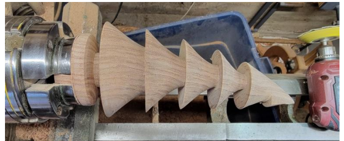
#12 Carve, sand, grind to form tip as desired.
